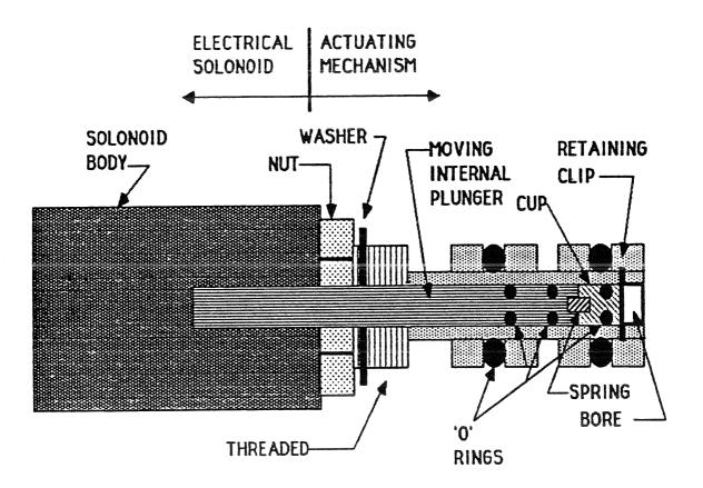
The 'O' rings required are easily obtained from any industrial bearing supplier in the yellow pages. The numbers given below are for Precision Rubber Products Co., Hartman Dr., Lebanon, Tenn. 37087. However, I believe the numbers are universal.
