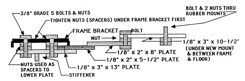
for the mount. You will need to grind away a little of the mount to prevent the solonoid striking the old crossmember bracket. With everything in place and tight you want to have 2" or less from the top of the mount to the rear adaptor plate to prevent the drive shaft hitting the tunnel. You will also have to make a new exhaust pipe mount.
